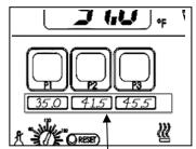
The stick-on strip fits beneath the controller's Preset Buttons. It is removable and reapplicable.
