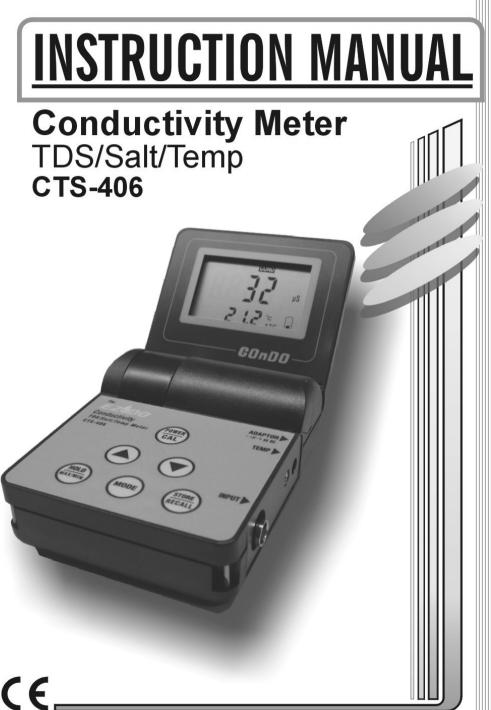
Thank you for selection CTS-406 Conductivity meter. It is possible to measure a wide range of Conductivity, TDS(Total Dissolved Solids), Salinity and Temperature with same electrode. We recommend that you read and follow the manual carefully.
