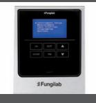
Front view of the viscometer, touch keyboard with 6 keys and graphic display.
