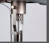
PT100 temperature probe is suitable adjusted by a clip which is attached to the spindle protector.
