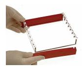
Casting dams allow gels to be rapidly cast externally while the unit is in use for gel running1
