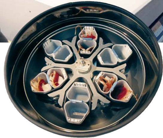
Image showing the rotor and double buckets for quad and triple blood bags of 500 and 800 ml.
