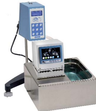
Immersion thermostat Digiterm controlling temperature of viscometer.
